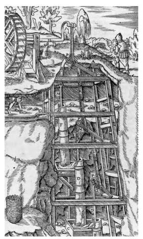
8.2 Hydraulic pump for mining operations. Woodcut in Georgius Agricola, De re metallica (On metallurgy, 1561). (Photograph courtesy of Sotheby's Inc., © 2003)
