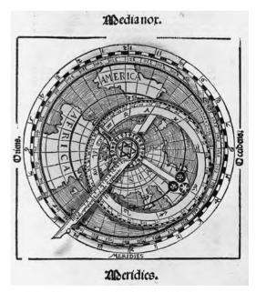
9.4 Movable navigational tool used to help determine a ship's position in the open sea. Woodcut device in the 1524 edition of Petrus Apianus's Cosmographia (Cosmography), 1524. (The device is called a volvelle and can be turned.) (Photograph courtesy of Sotheby's, Inc., © 2003)
